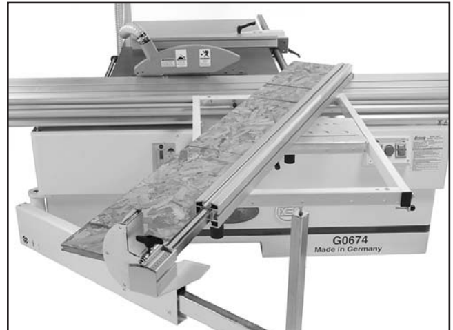
Figure 74. Example of miter cutting operation.
